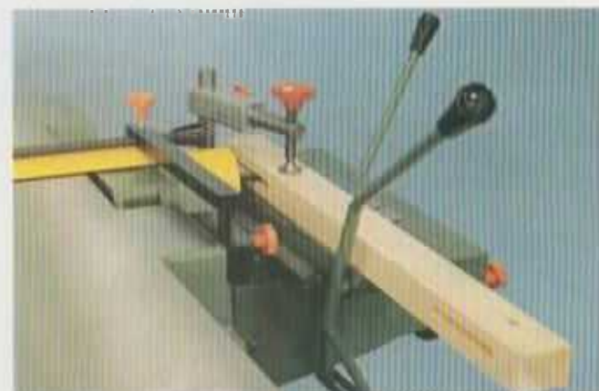
Mortiser. Independent rise and fall movement to the 19mm (3/4") capacity mortising unit longitudinal and traversal lengths and depth stops provided.
